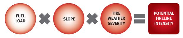
Figure 4: Method for calculation of potential fireline intensity.6
