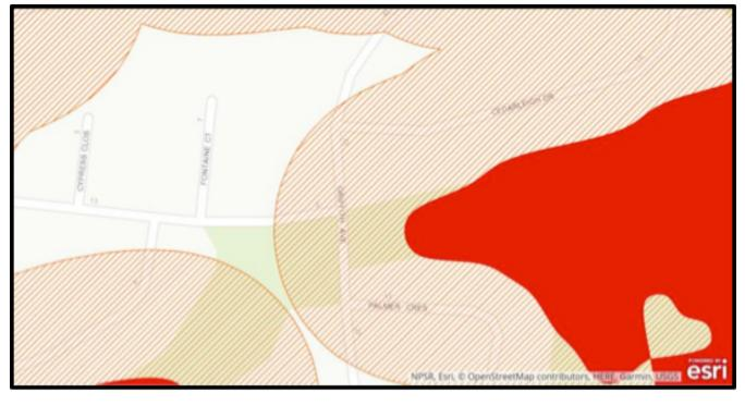
Figure 3: Example of a mapped bushfire prone area, including the potential impact buffer (land within 100 linear metres of mapped vegetation of greater than 4,000k/Wm fireline intensity). Source: SPP IMS
