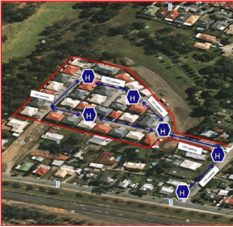
Figure 7 – Hydrant System design to minimum standards
