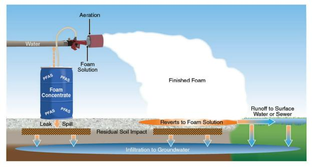
Plate 2 Release of firefighting foam (ITRC 2017)
